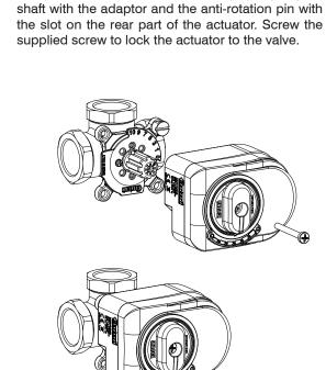
3. Apply the actuator onto the valve body by aligning the
